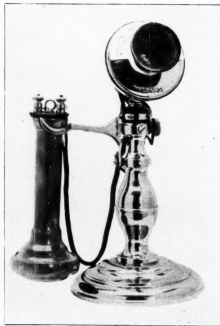
DESK TRANSMITTERS USED IN BANK.
