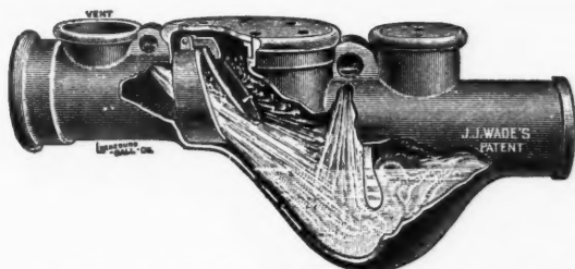
Main Trap in Cellar, showing Flushing Device in Operation.
