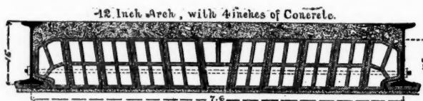
USED BY THE WIGHT FIREPROOFING COMPANY IN THE BOARD OF TRADE AND TELEPHONE BUILDINGS, CHICAGO.
