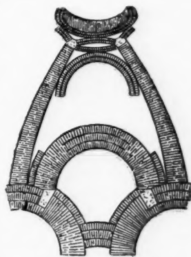
DETAIL OF CONSTRUCTION, CUPOLA OF PANTHEON, ROME.
