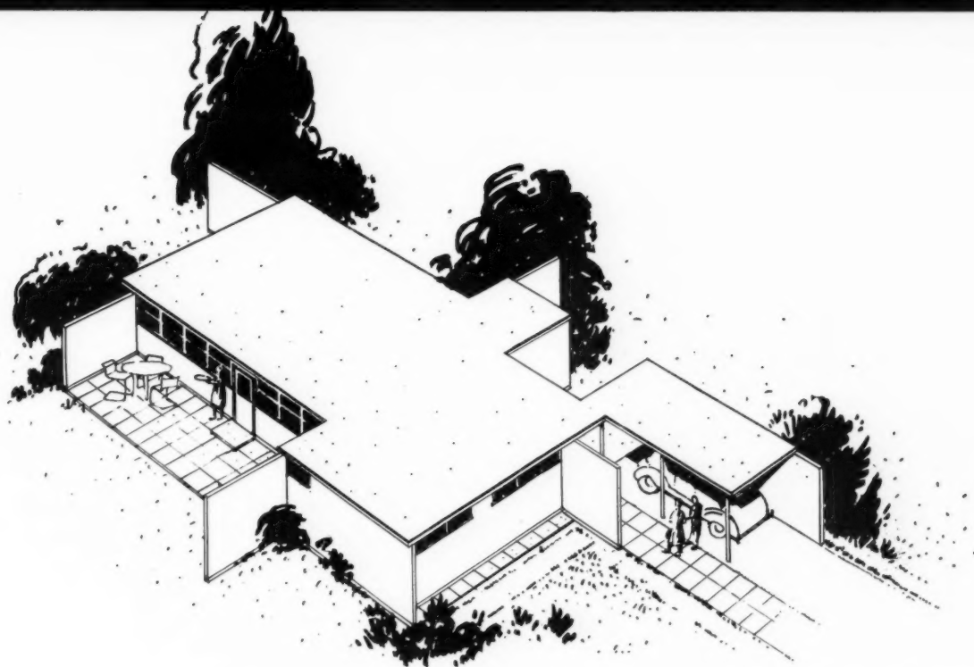
PERSPECTIVE VIEW OF A FIVE ROOM HOUSE, DESIGNED BY A. LAWRENCE KOCHER OF BLACK MOUNTAIN COLLEGE, N. C., SPONSORED BY REVERE COPPER AND BRASS INCORPORATED FOR PREFABRICATION AFTER THE WAR. ITS 36 WALL SECTIONS CONTAIN RADIANT HEATING TUBES AND BURIED PLUMBING CONNECTIONS. IT SHOULD SELL FOR $2,000.
