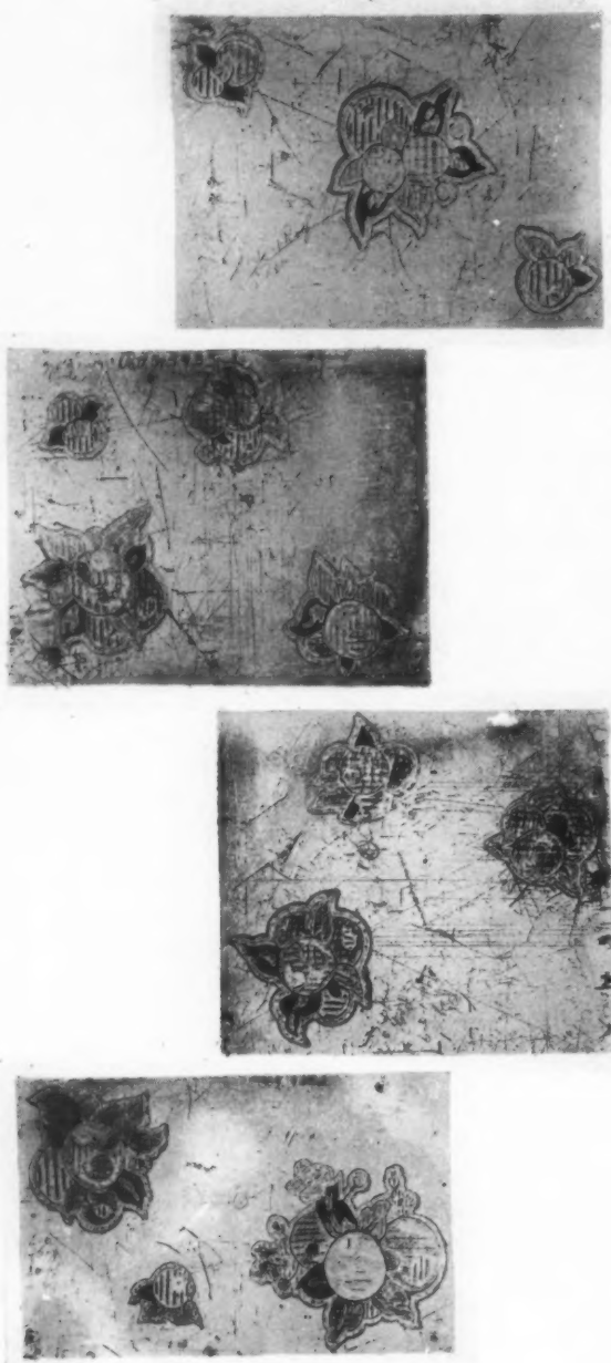
Reading from top to bottom: the four successive master zinc plates which guide the operation of the pantagraph machine in the engraving of copper rollers for a cretonne pattern. Each area of color is indicated by either stripes of the actual color or by solid color according to the character of the desired printing and these plates also carry the ground ruling which determines the amount or density of the color the rollers are to print.
