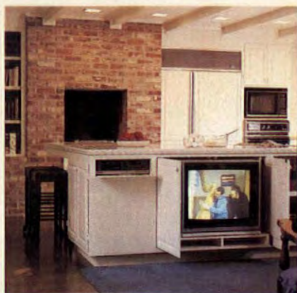
The television, concealed in the center island when not in use, pulls out on a swivel platform for viewing. A tape deck is hidden behind a pull-down drawer face.
