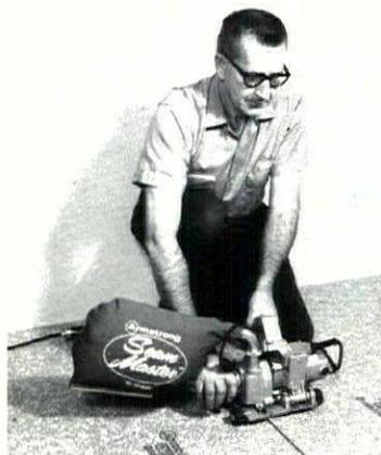
Seam cutter speeds floor laying, reduces fatigue, yet produces consistently even tight seams in sheet vinyl. Workman pushes tool across overlapped (no-pattern) flooring at 12' to 16' per min. A guide bar follows factory edge as 4" blade trims 1/2" from both edges. Armstrong, Lancaster, Pa.
