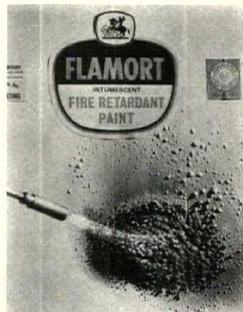
**Fire retardant paint** shields and insulates wood from flame, delays ignition. When exposed to fire, it bubbles and swells up to form a sponge-like insulating barrier, and it emits non-toxic fire-extinguishing gases that help to smother flames. After the fire is out and
