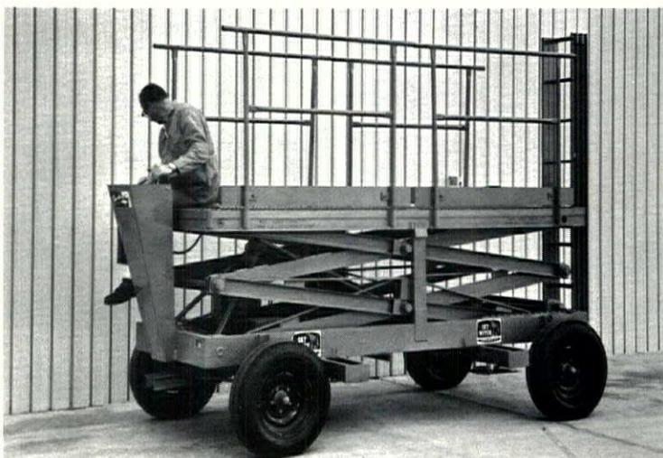
Mobile lift needs no tow truck, moves along with the job at up to 2 mph. Platform is 10'6" x 3'10", can be raised to a working height
