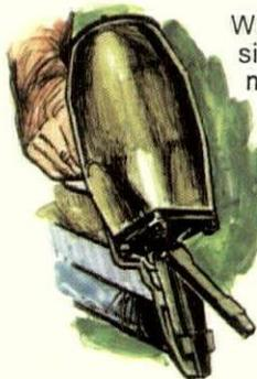
With the properly designed modern automatic tool, jamming is virtually eliminated. Bent fasteners are ejected instantly, automatically, and the tool is back in action with no delay.
