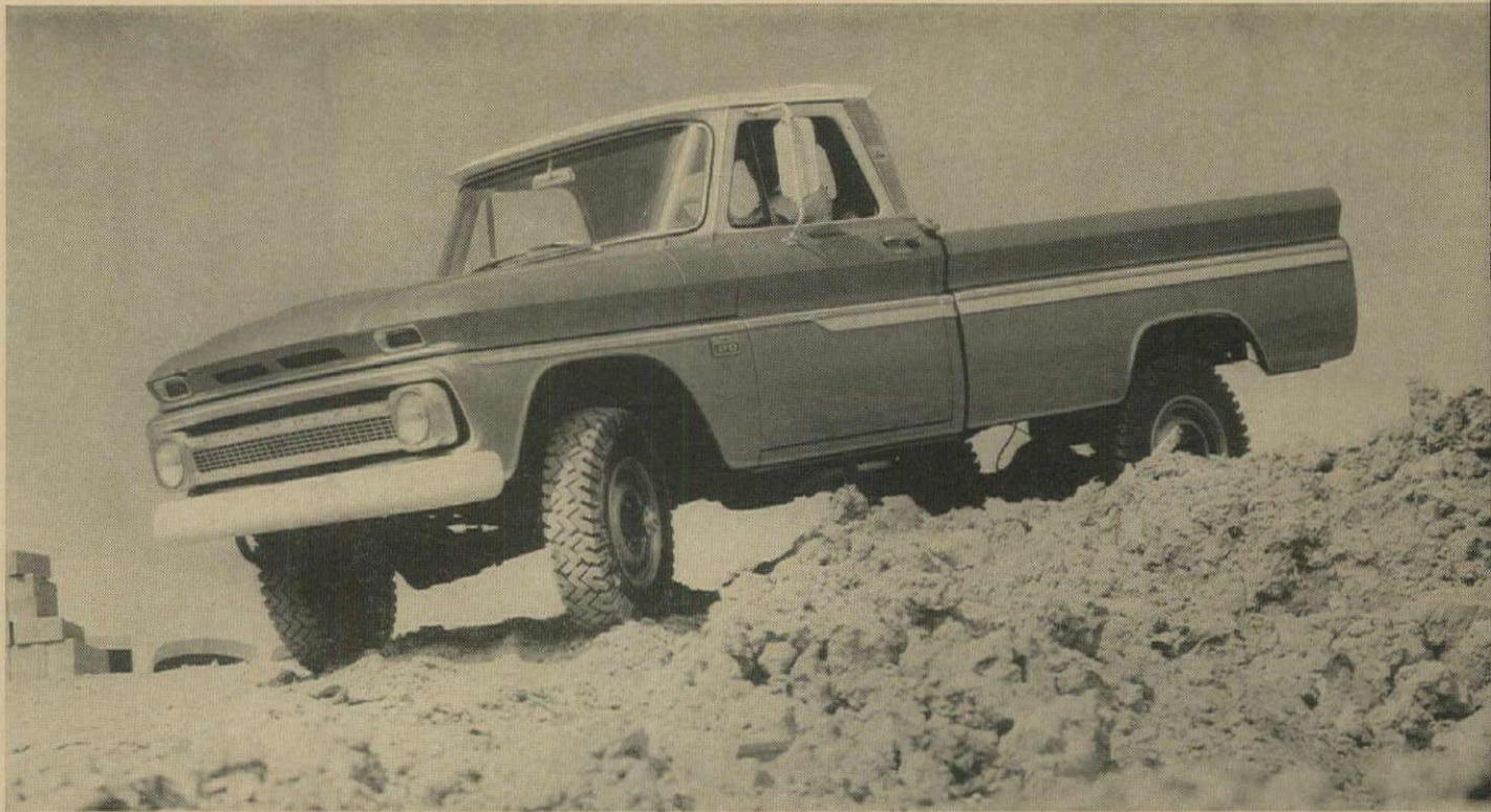
**Fleetside 4x4 pickups** are offered in two wheelbases, two weight ratings. Half-ton models come in 115" and 127" wheelbases with 6½- and 8-foot bodies. The ¾-ton model is an eight footer on a 127" wheelbase.
