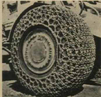
**Protective chains** for wheel tractors reduce tire wear in rocky soil by shielding tread and side walls from objects over 3" in diameter. Chains may be turned over for longer wear. Tire sizes: 33.25x35, 29.5x29, 23.5x25, 20.5x25, 17.5x25. Caterpillar, Peoria, Ill.
