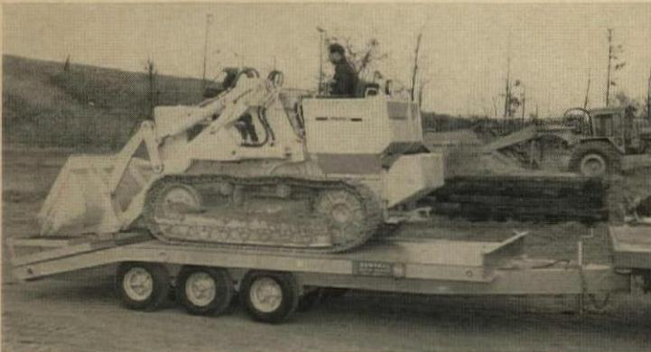
**Vehicle trailer** has spring-loaded ramps to speed up loading and unloading. Three-position tow hitch simplifies truck hook-up. Trailer shown carries 15 tons, other models range from 1- to 35-ton capacity. General Engines, Thorofare, N.J. (Circle 221 on Reader Service card)
