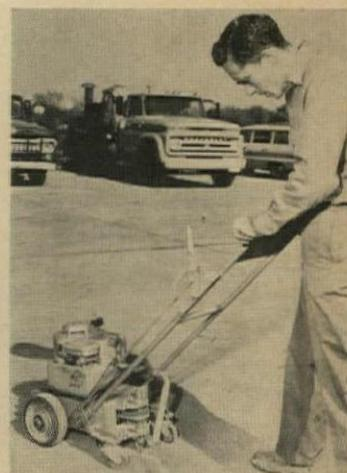
**Vertical router** widens and deepens random cracks in cement or bituminous concrete for proper sealing. Tungsten carbide bit, available in a variety of widths, cuts V-groove; engine exhaust blows out particles. Clipper, Kansas City, Mo.
