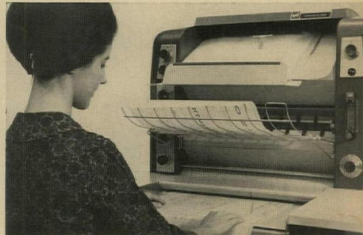
**Dual-roll diazo copier** has an electronic exposure computing device. Ozamatic 360 automatically selects the correct width diazo paper (up to 19") and cuts it to the length of the original. General Aniline, Binghamton, N.Y. (Circle 235 on Reader Service card)
