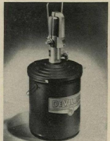
**Small airless pump** to cut overspray in medium production will handle all conventional paints with a standard airless gun and a compressor as small as 1 hp. Pressure is supplied by a chromium piston in a stainless steel cylinder, operated by an air motor. Price: \$192.50 FOB Toledo.
