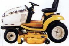
Cub Cadet's GT 2554 has a 54-inch cutting deck with a system that uses blasts of air to help lift grass for a cleaner cut. You can cut in reverse, and the heavy-duty drive shaft transmission allows for a smooth ride. \$4,000. cubcadet.com.
