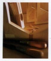
2. The entire table is constructed using the time-honored technique of "biscuit joinery." No nails or staples are used at all.
