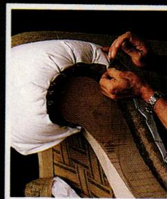
A hand-filled down pad is pinned over a scroll arm.
