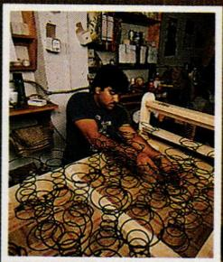
Springs are anchored and adjusted to create a level surface.
