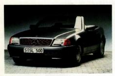
A long hood, steeply sloping roof pillars, a compact roof, and integrated headlights and taillights are all part of the Mercedes SL's aggressively aerodynamic new design.
