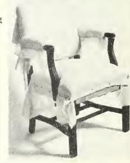
Cut burlap 2 inches larger than seat frame. Attach with #6 tacks around frame. Tack edge rolls to sides and front, keeping flush to outer edge of frame. Cut rubberized hair 34-inch thick to fit chair seat and cover edge rolls. Stitch in place. Add 2 layers cotton batting extending over seat to underedge of chair. Measure muslin to cover entire seat. Tack under frame. Trim excess.
