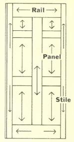
Arrows show how wood grain runs in panel door; Blanks can be vertical or horizontal.
