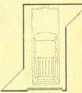
Garage is 10' x 20', with added triangular wings: total, 225 sq. ft. For complete building plans and list of materials, write Department W-1, Oldsmobile Div, Lansing, MI 48921.
