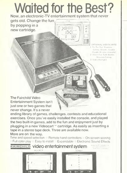
GAME CONSOLE: Based on the Fairchild's F8 microprocessor, the console comes with hockey and tennis built into its memory. The digital hand-controllers provide 8 directional movements, +/-- [x, y, z,  $\mathbf{e}$ , ], for the utmost in maneuverability. For example, in hockey, the forwards roam the ice in the x and y coordinates, their sticks rotate in  $\mathbf{e}$ and the goalies guard their z-coordinate goal line.
