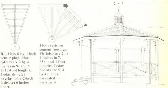
laths, and the 8 ridges covered with a screwed-on metal capping strip. The cupola should also be built on the ground and hoisted into place. It consists of a sheet-metal (galvanized flashing) roof, painted to simulate copper, atop 8 6-by-16-inch shutters of the indoor type. Final step, of course, is to paint exposed surfaces—except shingles and flooring—in whatever colors suit you.
