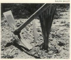
Part mattock, part grape hoe, this superbly balanced tool is light, sharp, has a 4-foot handle, and is capable of precise handling.
