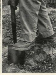
A spade is a spade. Old model, above left, has too thin a blade for an instep, so massive shaft is fitted with a special foothold. Modern spade, above right, takes a heavy foot on its shoulder.
