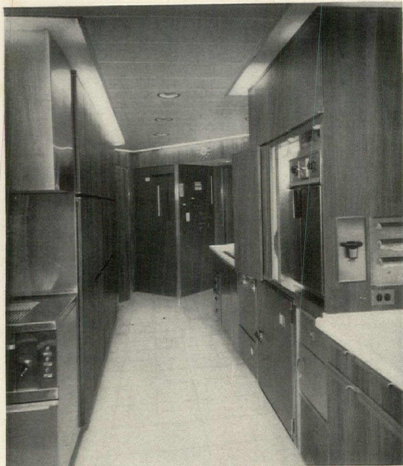
Light strips bordering the ceiling throughout the kitchen give general illumination; spotlights and under-cabinet fluorescents light working areas.
