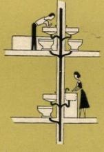
Cut plumbing costs by placing bath, kitchen, and laundry back to back or above one another to reduce number and lengths of pipes and soil lines.
