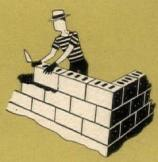
Concrete block used for foundation and above-grade walls is definite economy. Use exposed face of block, painted or left natural, as interior wall finish.
