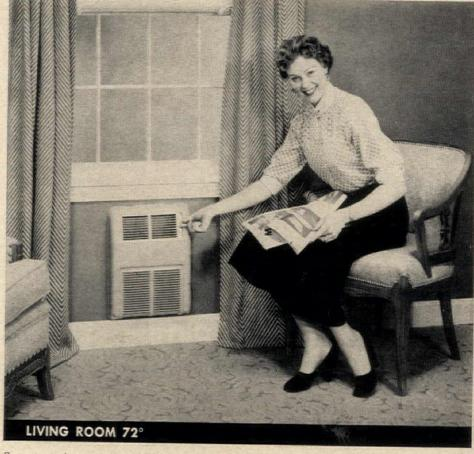
Compact room heaters, only 18 inches high, are recessed into walls, with only grille projecting. Can be painted to fit any color scheme. Three sizes: 6,000; 12,000; and 18,000 Btu. 12,000 Btu. size shown above.
