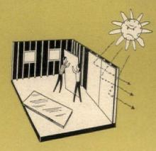
Double-purpose wall materials, available in large panels, serve as interior wall facing, have reflective backing to keep sun's rays out of house.
