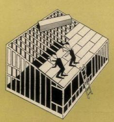
Multi-purpose roofing saves labor, acts as sheathing, insulation and interior finish. Should be used on a low-pitched or flat roof. It is then covered with layers of felt, asphalt.
