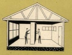
Prefabricated roof trusses eliminate interior bearing partitions, allow open plan. Storage walls between rooms replace partitions, are sound deadeners.
