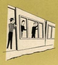
Prefabricated wall sections save time, money and are easy to install; come complete with doors, windows, insulation, inside and outside finish.
