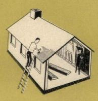
Insulation with vapor barrier cuts down on fuel bills, keeps walls dry, house warm. White paint or finish on a roof deflects sun's rays in summer, keeps all interiors cooler.
