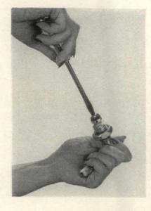
4. Turn the spindle upside down and grip it tightly in one hand, or with a pair of pliers. Using an ordinary screw driver, remove the protruding screw at the end. This holds a small rubber disc, called a washer, which is usually the seat of the trouble. Take care not to damage the threads.
