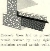
remain warmer by using rigid insulation around outside walls.
