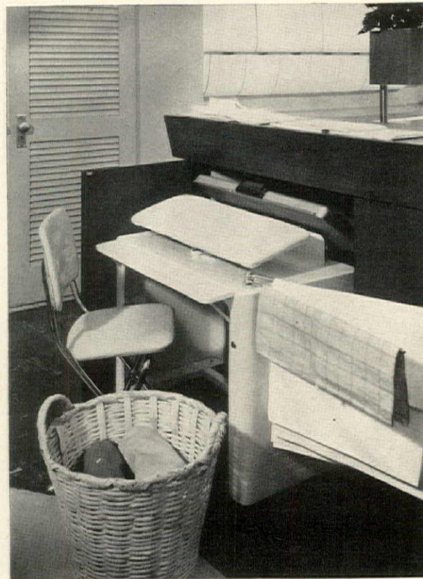
Above Ironer with "Toe-Touch" control is concealed in corner of U-shaped island, slides out easily. Bars swing to hold ironed linens.
