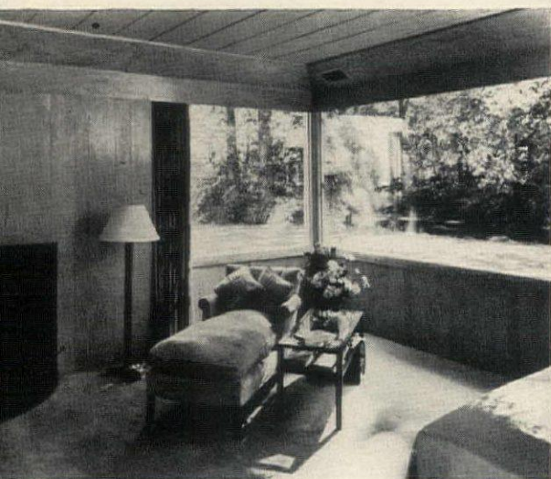
Louvered ventilating panels below windows bring draft-free air into the bedroom.
