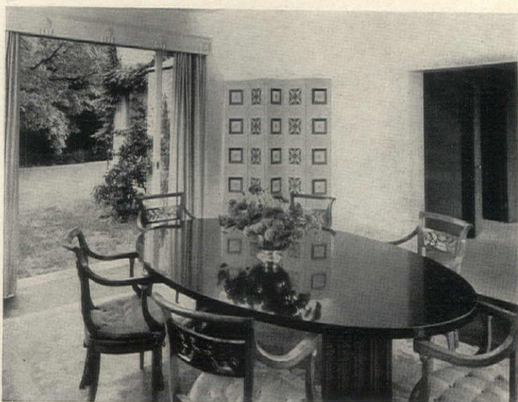
A glass door, seven feet wide, slides on tracks into the adjacent wall. In summer weather, it transforms the dining room into an airy pavilion.
