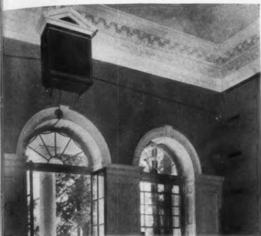
**The seven-day clock**, designed by Jefferson and built in the workshop of Monticello, has cannon-ball weights which show the day of the week as they move down the wall.
