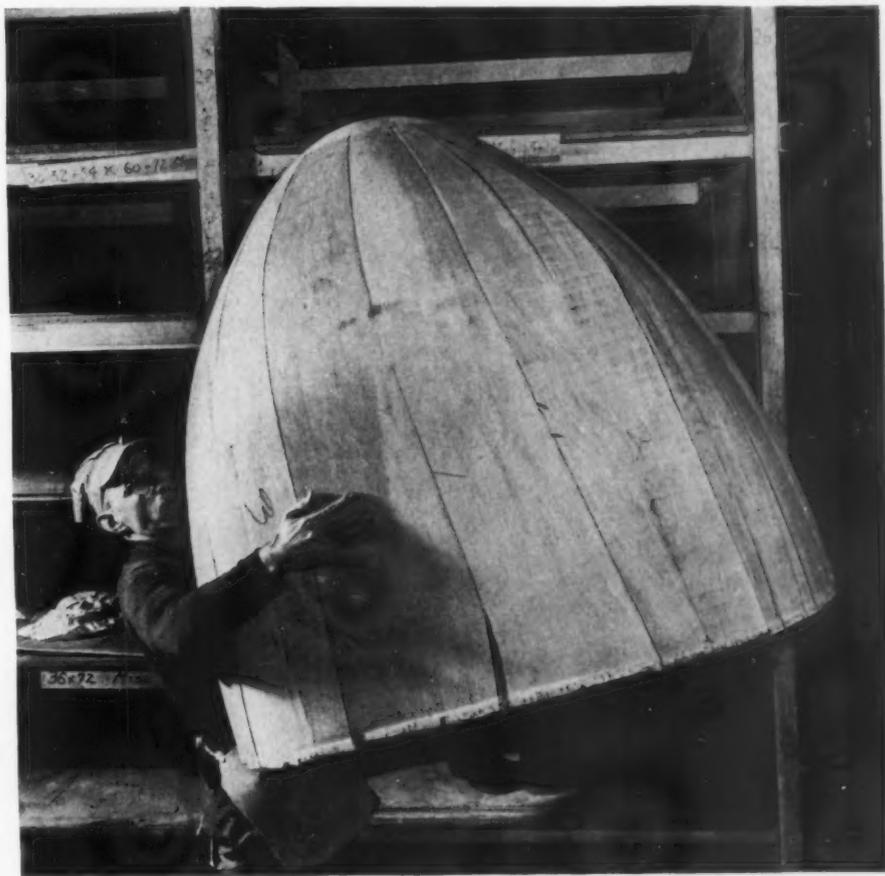
Waterproof plywood is raw material for most of G. R. I. program, is made and shaped locally by Haskelite. Amazingly light, Haskelite plane nose can be carried by one man; see above.
