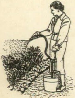
After the hand sprayer, used only indoors, the simplest is the pump inserted in a bucket. Suitable only for a small place
