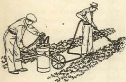
Two-man sprayers, suitable for large places, hold a long supply of disease-resisting mixtures. Keep all the parts clean
