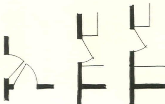
Kitchen Doors. BAD (left): Doors strike if swung simultaneously. BAD (center): Swings too near work space. BETTER (right): Door swings clear
