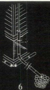
6. Downspouts should be fitted into a cast iron pipe 18 in. above grade. This carries the water below frost line to a tile drain leading from the foundations to a dry well or natural outfall. 7. Porch steps should be of decay-resistant wood, set on their own foundation, and freely ventilated at the side. No woodwork should be in contact with the ground. 8. Insulated floor above unoccupied basement. Note permanent ventilation and copper termite shield under sill (cf. illustration at right)
