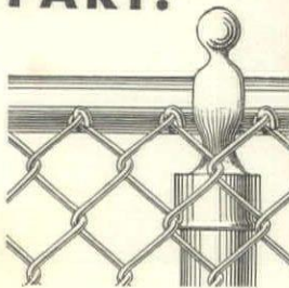
ALL POST CAPS FIT DEEPLY OVER THE POSTS TO KEEP OUT MOISTURE.
