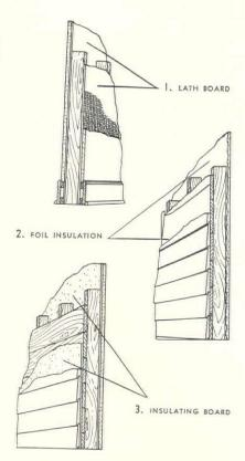
WHILE many of the manufacturers make more than one type of insulation, we have selected typical examples. "Foil" insulation reflects heat from a highly polished surface. 1, The Celotex Co., Inc.; 2, Reynolds Metals Co., Inc.; 3, Insulite Co.
