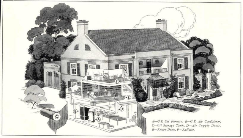
One way of modernizing an old house with G-E Air Conditioning. Notice that ducts supply the ground floor, while the upper floors retain the radiators of the existing heating system.
