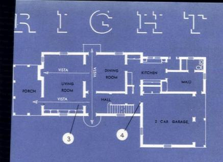
**General plan.** Wrong: Exterior walls and roofs are too broken up (2); partitions and walls fail to carry through in straight lines; roof will invite leaks; living room is not much more than a passage way (1). Spend plenty of time going over general scheme of plan and thereby save more than all the squeezing of size and equipment after estimates are received
