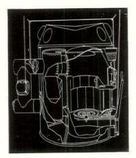
Steel furnace equally suited to coal or oil. The suspended bell protects the crown from direct heat. L. J. Mueller Co.
