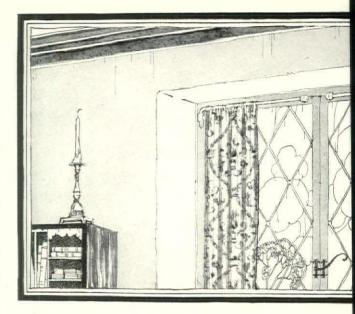
A popular treatment for casement windows consists in hanging curtains from hinged brackets which swing back leaving the opened window free and swing the curtain from exposure, Brackets from H. L. Judd Company, Inc.
