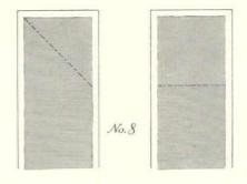
In seaming carpets, two methods are used. Note the difference in mitering and butting. (Right) Butting adds to the life of a carpet and looks better
