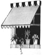
Above is a scalloped valance of painted tim. When the awning is rolled all the way up it is completely concealed and protected by this shield
