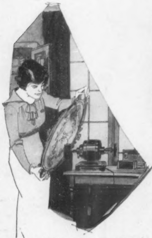
A general utility motor will turn the buffer, the knife sharpener, and, in some cases, can be used for freezing ice cream and doing other kitchen odd-jobs
