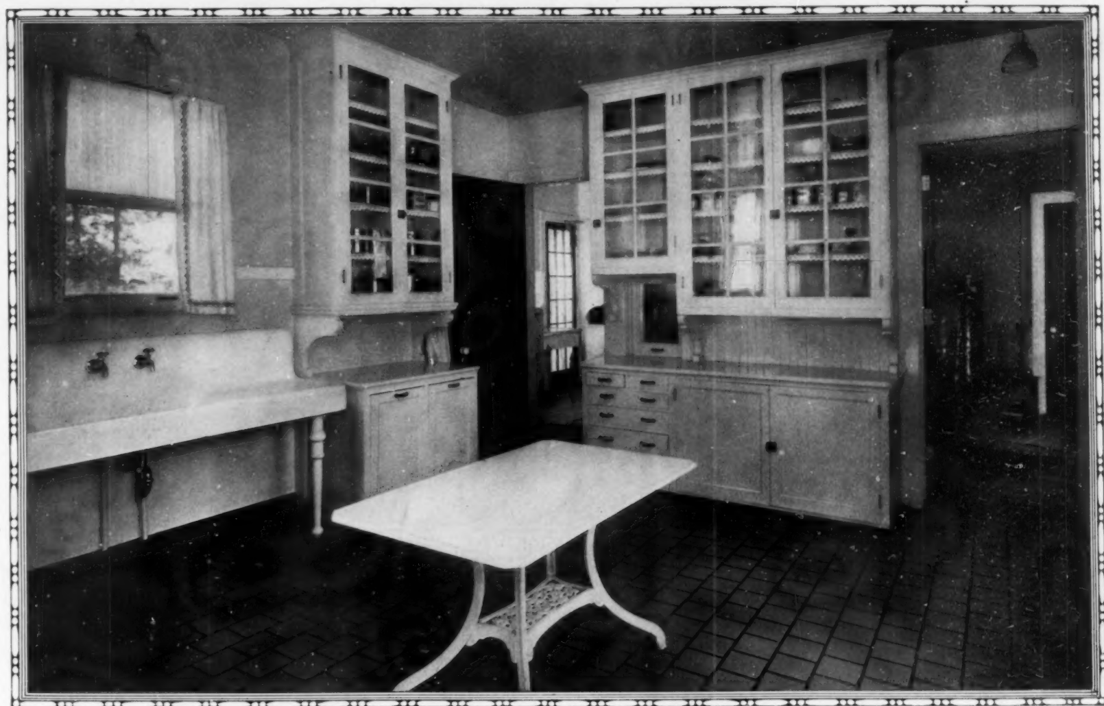
A good kitchen for a larger family. Size, type and location of sink are excellent. Note light over sink. There is the proper relation of table, sink and counters one to the other and to pantry. The floor is covered with inlaid linoleum and the walls painted
