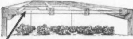
Between the two layers of glass is a 1/4 inch blanket of dry, still air. Being transparent, this layer permits the plants to get all the light all the time. Glass slips in and is held securely without putty. Easily repaired.
