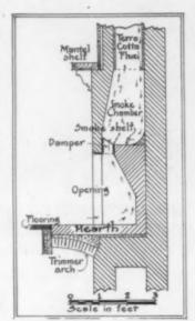
This vertical section through the center of a fireplace shows the scientifically correct form for maximum efficiency and
