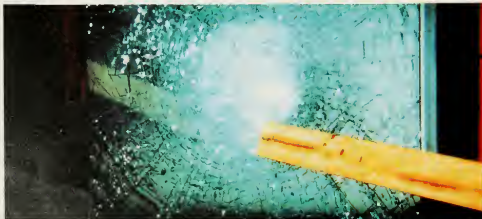
The Point of Impact: A nine pound 2 x 4, shot from a test cannon at 50 feet per second (34 mph), impacts a window system utilizing impact-resistant glass. The window, working together with the interlayer, resists the 2 x 4, preventing it from breaking through the glass.
