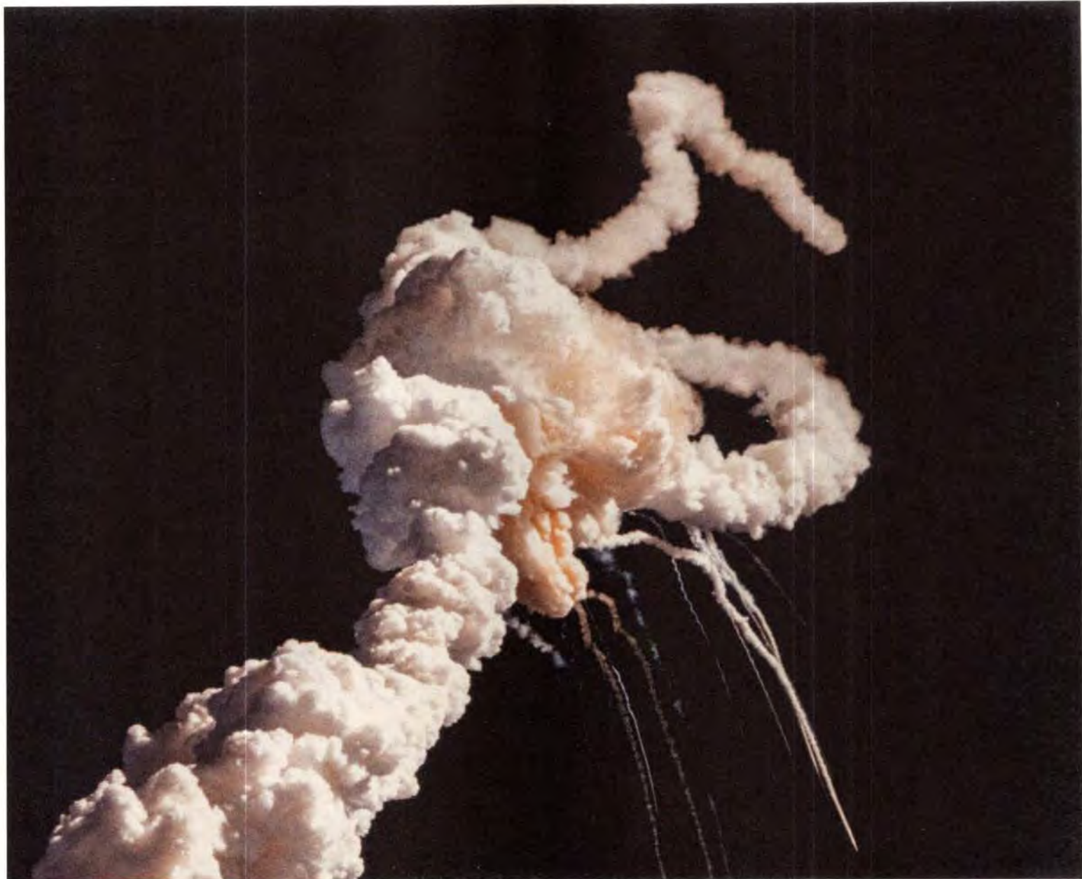
On January 28, 1986, the Challenger space shuttle and her seven-member crew were lost when a ruptured O-ring in the right solid rocket booster caused an explosion soon after launch. Image © NASA (86-HC-220)
