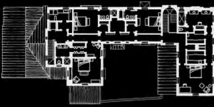
House 4 Second and first floor plans. The circulation, informal downstairs and formal upstairs, wraps around the central courtyard.
