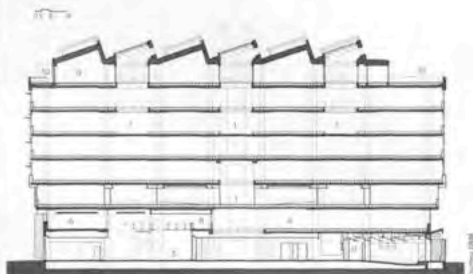
Longitudinal section through the UT School of Nursing Building, showing location of roof garden and three interior atria.
