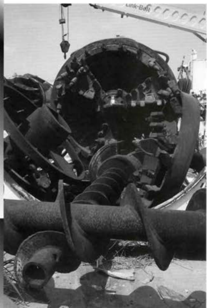
Big bore: Microtunneling machines such as the above, seen in pieces at a contractor's yard, are used to carve paths through Houston's clay for sewage and water lines.
