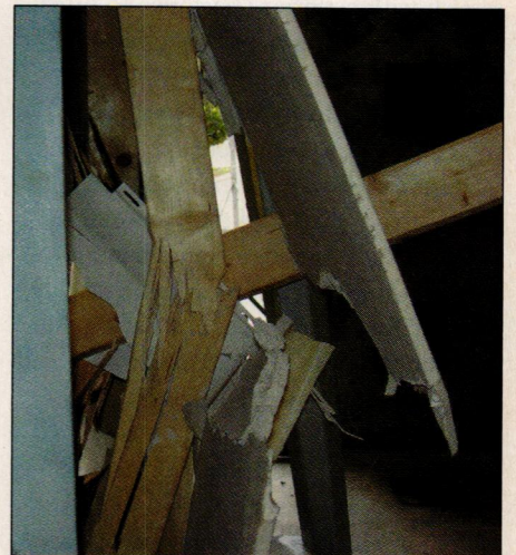
FIGURE 1. Windows that meet the ASTM E 1886 and ASTM E 1996 impact standards shatter but do not present an opening that will either pressurize the interior or allow undue amounts of water into the home (above). However, most conventional wall systems do not fare as well under the same test. A typical vinyl-sided wood-frame wall is obliterated by the large missile test (right). A concrete block wall performs a bit better but still allows a sizable hole for wind and water to penetrate (top right).
