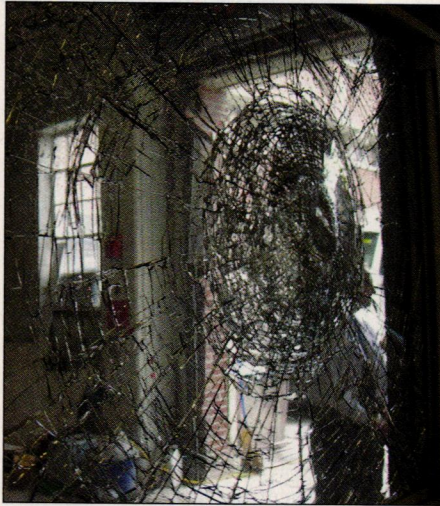
FIGURE 1. Windows that meet the ASTM E 1886 and ASTM E 1996 impact standards shatter but do not present an opening that will either pressurize the interior or allow undue amounts of water into the home (above). However, most conventional wall systems do not fare as well under the same test. A typical vinyl-sided wood-frame wall is obliterated by the large missile test (right). A concrete block wall performs a bit better but still allows a sizable hole for wind and water to penetrate (top right).
