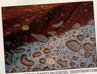
FIGURE 3. The reason boat owners love spar varnish is shown above: a deep, rich, clear coat that repels water and reveals all the beauty of the wood. A finish like this takes 10 to 12 coats, however, and needs continual attention to maintain its good looks. Without a yearly sanding and refreshing, varnish fails by yellowing and peeling (right). When that happens, it's time for sanding back to bare wood and starting over.
