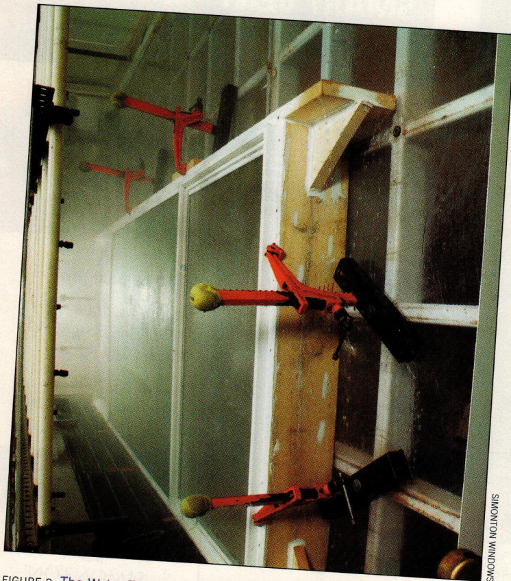
FIGURE 8. The Water Test: To meet AAMA minimum water penetration rating, a sample window is subjected to a negative pressure equal to 15% or 20% of the design pressure across the inside of the test assembly. The window exterior is then hosed down with a rack of water jets that is equivalent to a rainfall of 8 inches per hour. If any leakage occurs on the interior, the window does not pass.
