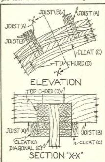
minimum of cost and is generally fabricated at the building site, being built up of small dimension lumber as shown in the accompanying sketch.
