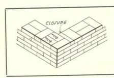
Fig. 2. Flemish bond with single header and one stretcher. Two ¾ brick are used on corner and a closure piece of a half brick split lengthwise
