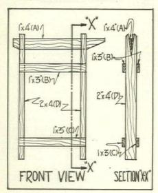
The saw will then be found to be held firmly and will stay so until the 1"x4"s (A) are taken out of the notch. The clamp may be set up anywhere and nailed to any convenient wood column or any stable object in order to hold it up-
