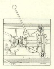
The Warford Heavy Duty is mounted in a universal joint forward; the weight of the unit and torsional strains of power take-off operation are absorbed by the sturdy cross-member which also reinforces the Ford frame.
