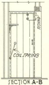
swing panel rounded out in the edge on both sides. When the door is opened this panel strikes the soffit of the attic stairs, but does not stick because of the rounded edge. As it opens in it allows the door to open all the way. The coil spring closes the door and when the panel strikes the door stop it closes back in place.-P. A. Hall.
