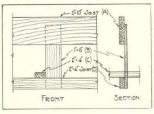
mid-point, where the deflection is bound to be greatest, a piece of 1"x6" (B) is nailed to the ceiling joist (D) and to the roof joist (A) so that the joist (D) is really suspended from the joist (A). This will increase the stiffness of the ceiling to a great degree. The stiffness may be further increased by a cross strip (C).
