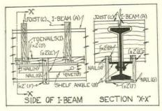
essity for maintaining a given elevation, or in an effort to conserve wall height; at any rate some provision must be made for attaching the lath to the beam in order to hold the plaster.
