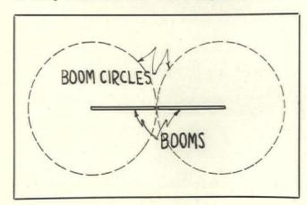
Fig. 4. By taking up and paying out the proper guys these derricks may be shifted as the work advances
