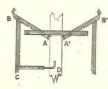
SHOWING METHOD OF ATTACHING TO POLE—set spurs A, A1 level, then pull down arms B, B1, adjust brace C in place and tighten hand screw D. Weight 10 lbs. Folds to very small space.
