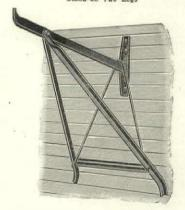
Stucco Brackets Attach to Wall With 4 Nails
