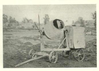
Fig. 1. This small tilting mixer is well adapted to small work where portability is the big item
