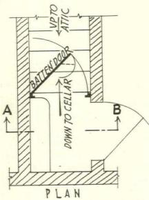
a door can be hung to shut out the dust. This door would have to open out over the stairs, and would ordinarily strike the soffit of the stairs to the attic.
