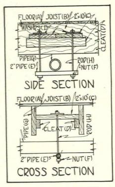
(D) short sections of joists should be set to form a shelf.
