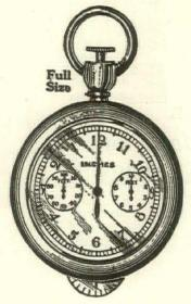
Map Measure, watch pattern. With device to set at zero by pressing knob shown in illustration. Large circle records inches and ½ inches. Second circle records feet up to ten feet. Beyond ten feet, the number of feet up to 100 feet is recorded on the third circle. Useful for Architects, Engineera and Contractors for taking dimensions from plans. The measurements are recorded full size and then simply multiplied by the scale in which the drawing is made. Very accurate. Postpaid, each, \$4.50 net.
