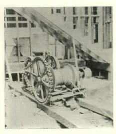
Fig. 1. Here the engine runs continually, revolving the clutchoperated winch. It is mounted close to the drum to accommodate the chain drive
