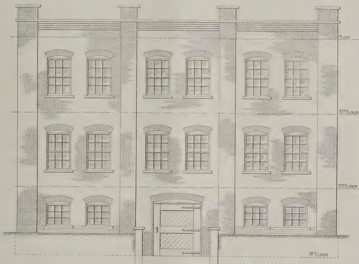
A Plan for a Small Factory Building—Fig. 1, Front Elevation—Scale \frac{1}{8} In. to the Foot
