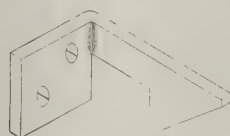
Fig. 16.—Perspective of Metal Catch for Back of Drawer Shown One-Half Full Size
