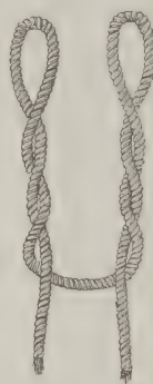
Fig. 8—A Better Method of Arranging the Rope
