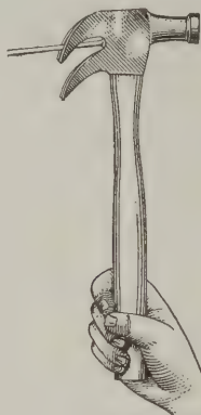
Fig. 7—Double Claw Hammer in Process of Starting a Nail
