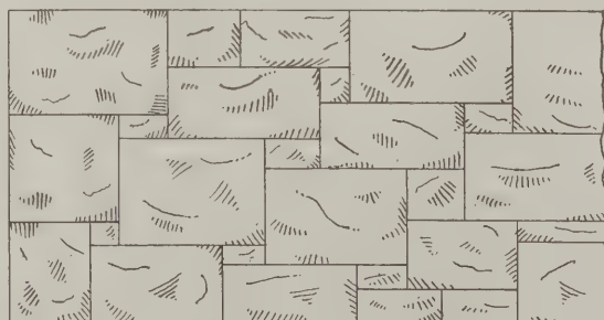
Question in Masonry—An Example of Step-Work
