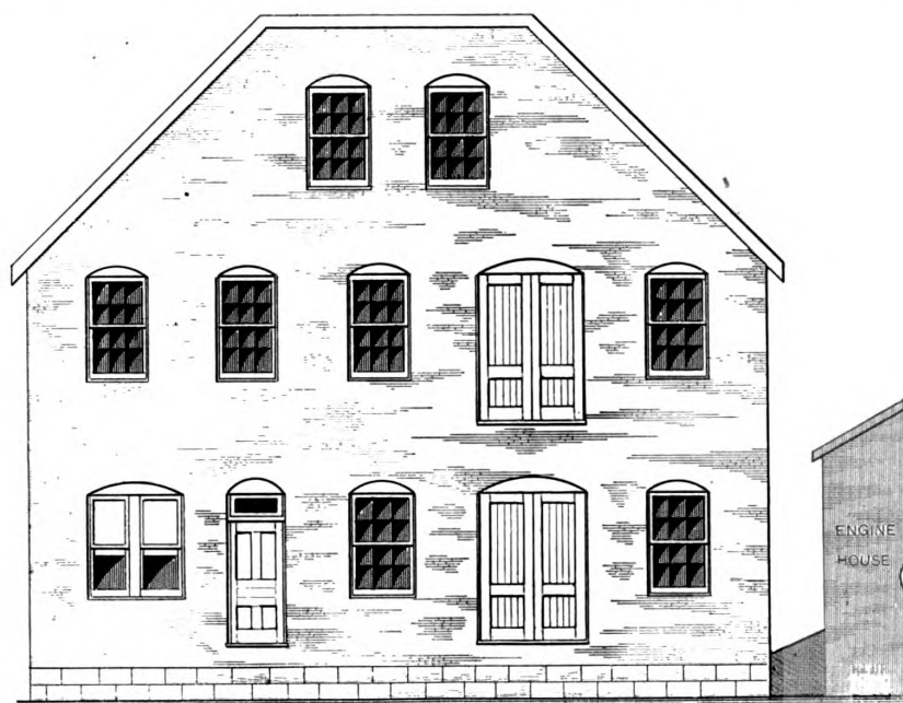
Front Elevation, Showing Portion of Engine and Boiler House at the Right.—Scale, 3/32 Inch to the Foot.
