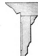
Window Stool and Apron. Scale, 3 Inches to the Foot.
