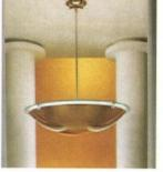
disk with one side frosted. Four machined aluminum grip blocks with a brush finish support the green disk, while gripping the spun dome. A single aluminum center stem, also with a brush finish, completes the product. The light source is a 6-26W quad compact fluorescent using electronic integrally mounted ballasts.
