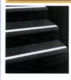
Musson's Glo-Strip stair treads are photoluminescent (glows in the dark). A 2" wide white grit-strip made with non-toxic, non-radioactive zinc-sulfide crystals absorbs and stores light, then releases this light energy over a period of time. The Glo-Strip luminescence can be seen after lights cease operating which helps lead the way to safety. Recharge by exposing to light for a few minutes. Meets ADA slip resistance and high
