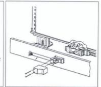
Patented Product 180° swivel mount base feed solves field installation problems
