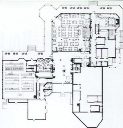
The 125-seat Starbuck Restaurant at Harbor View Hotel (left, top) features dark mahogany and cherry wood finishes blended with light bleached woods to create contrast and depth. Columns recalling Victorian-style architecture were added. Easily accessible from the hotel lobby, FORMA also added a new exterior entry, allowing local patrons to enter the restaurant without passing through the lobby.
