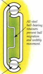
Steel or polymer ball-bearings are available to provide slide
