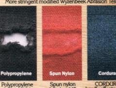
failed at 445 double rubs. failed at 164 double rubs.
