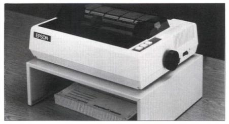
Tabletop printer stand from Tiffany Stand and Furniture Co. enables small printers to be placed on worksurfaces. Construction is of heavy gauge metal with two, grommeted paper feed slots; one slot is centered and the other is located near the rear edge to accommodate both bottom- and rear-feed printers. Available in putty- or black-baked enamel, product includes paper guides, footpads, and vibration damper pads. **Circle No. 384.**
