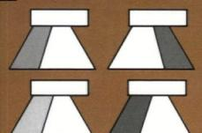
adjust <sup>€</sup>VARI-GRID<sup>™</sup> diffuser to provide the desired light intensity.
